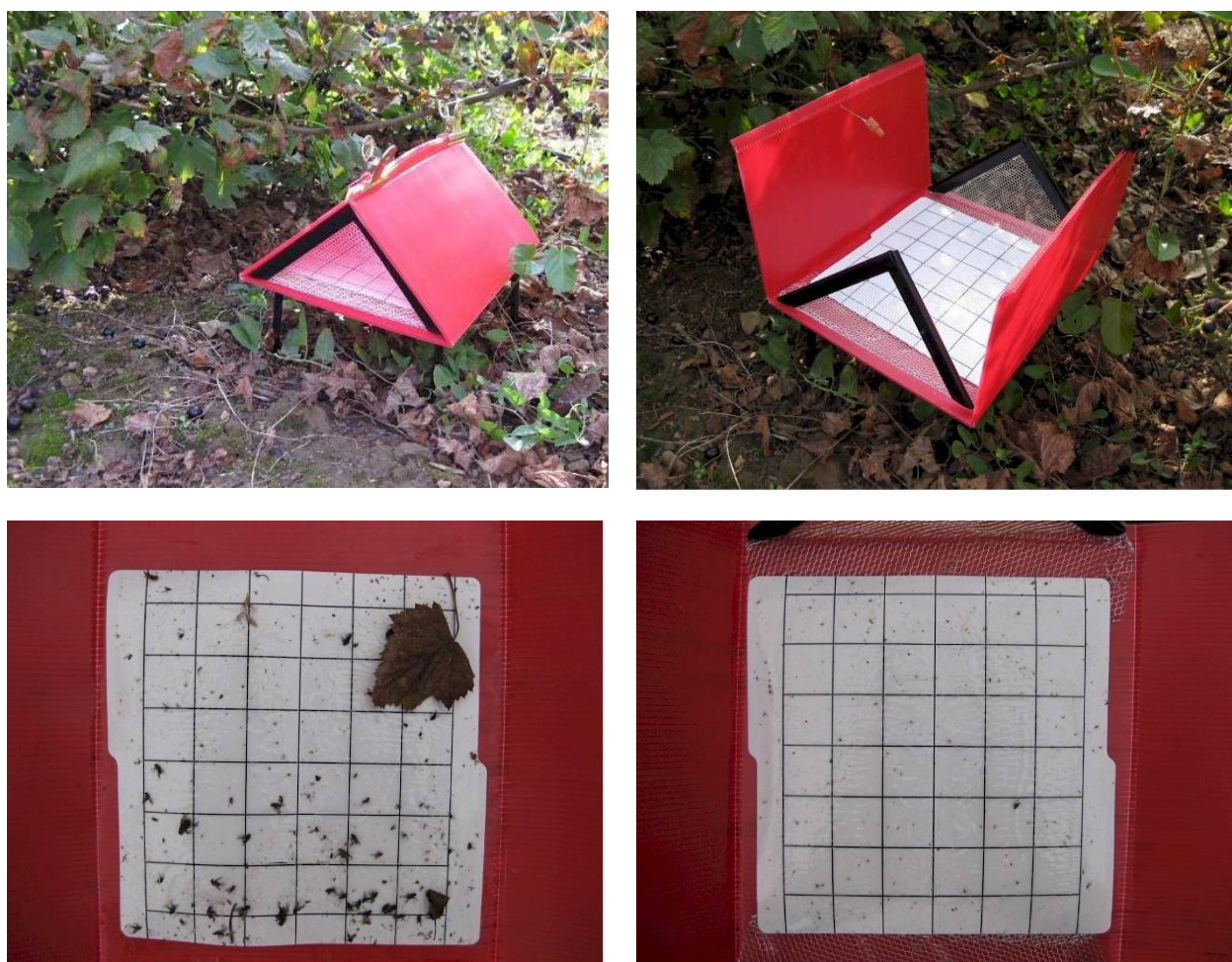
Figure 6.1. Prototype blackcurrant leaf midge sex pheromone monitoring traps in operation (top left), opened to change sticky base (top right). The sticky bases from traps deployed for 2 weeks in early September at East Malling Research without grids at entrances (bottom left) with grids at entrances (bottom right).
